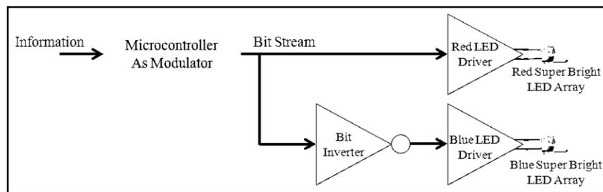
Figure 2. Complete VLC Modulation System Design
